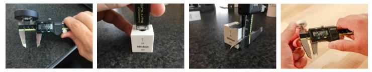
The internal measuring faces on many styles of calipers use crossed knife-edges. Due to the thickness of the faces and the clearance between them, additional errors can occur when measuring small internal diameters. For calipers that utilize cross knife-edge measuring faces, ASME B89.1.14 requires an additional test using a 0.2 in (5 mm) diameter ring gage for all calipers with measuring ranges up to 12 in (300 mm).
