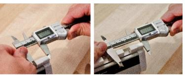
Testing near the tip of the jaws...and close to the beam
